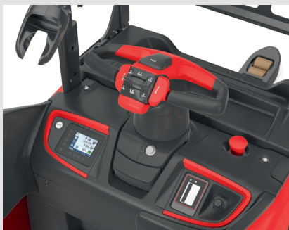
Ergonomic, height-adjustable tiller
